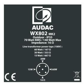
When the loudspeaker is connected to 70.7V facilities, the power indicated in the image on the previous page will be reduced to half the power, and when connected to 50V facilities, the power will be reduced to a quarter.
